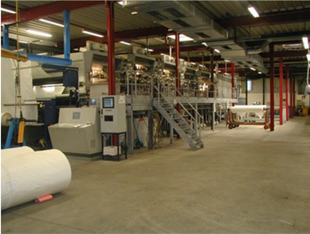
Fig. 2: Photo of the continuous washing machine for polyamide fabric at Global Safety Textiles Limited in Murg
