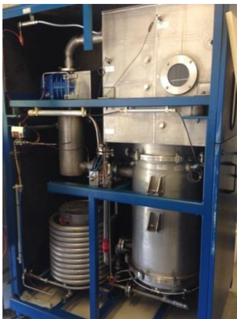
Fig. 9: The milky concentrate from the nanofiltration plant is de-watered under vacuum in an evaporation plant provided by H 2 O Ltd. in Steinen/Germany
