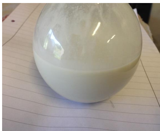
Fig. 8: Milky concentrate from the nanofiltration plant which is subsequently evaporated under vacuum
