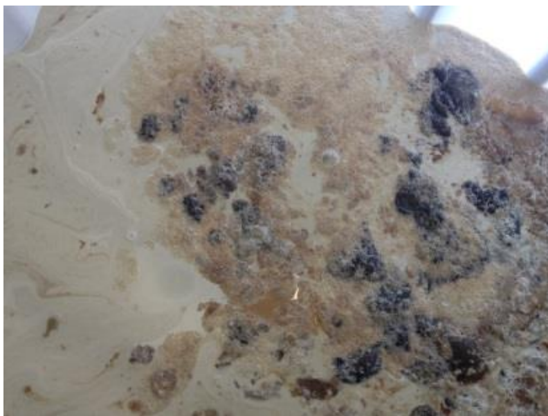
Fig. 10: Photo of the concentrate after evaporation with a water content of 3 -5 % which is collected in intermediate bulk containers (IBC) for external disposal (incineration)
